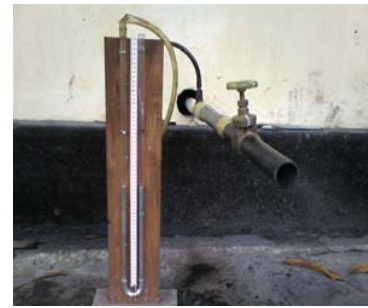
Fig 2. Arrangement of mercury manometer to measure exhaust backpressure.
